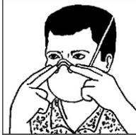
4. Place your fingertips from both hands at the top of the metal nosepiece. Using two hands mold the nose area to the shape of your nose by pushing inward while moving your fingertips down both sides of the nosepiece. Pinching the nosepiece using one hand may result in improper fit and less effective respirator performance. Use two hands.
