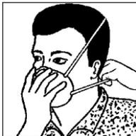
3. Position the respirator under your chin with the nosepiece up. Pull the top strap over your head resting it high at the top back of your head. Pull the bottom strap over your head and position it around the neck below the ears.
